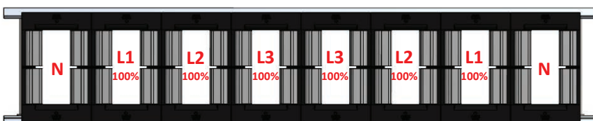
Optimized Conductor Arrangement (Load current balanced)
